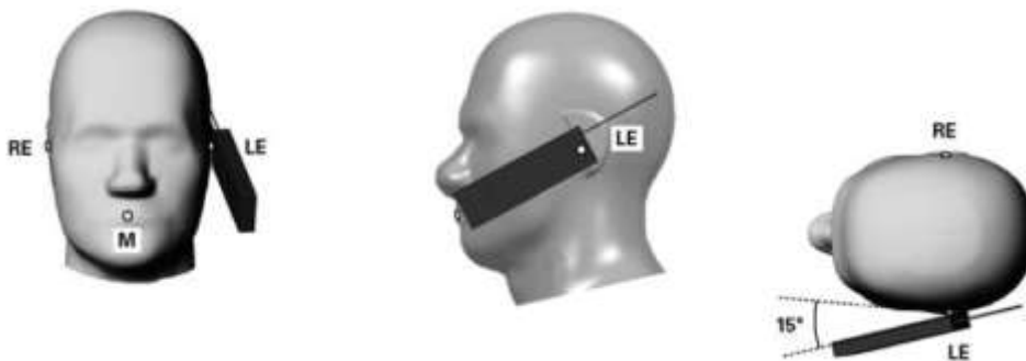
Figure 6.5. Tilt 15° position of the wireless device
