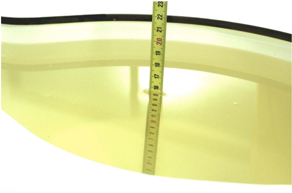
Picture 7-10 Liquid depth in the Flat Phantom (2600MHz)
