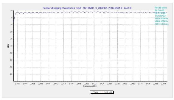
Fig.96. Number of hopping frequencies:  $\pi/4$  DQPSK, Channel 0 - 39
