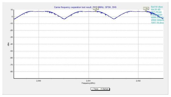
Fig.91. Carrier frequency separation measurement: GFSK, Channel 39
