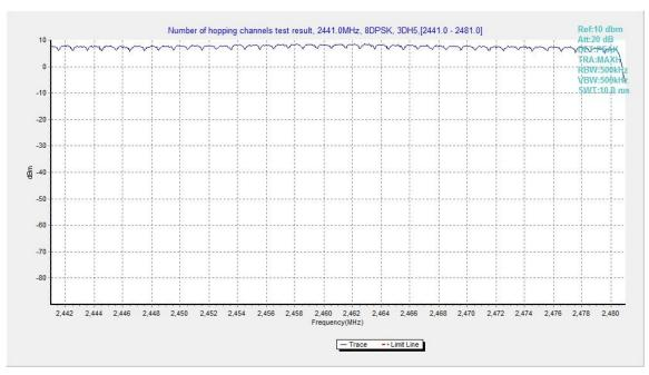
Fig.99. Number of hopping frequencies: 8DPSK, Channel 40 - 78
