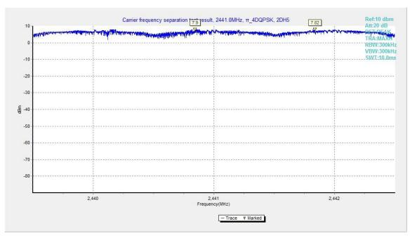
Fig.92. Carrier frequency separation measurement:  $\pi/4$  DQPSK, Channel 39
