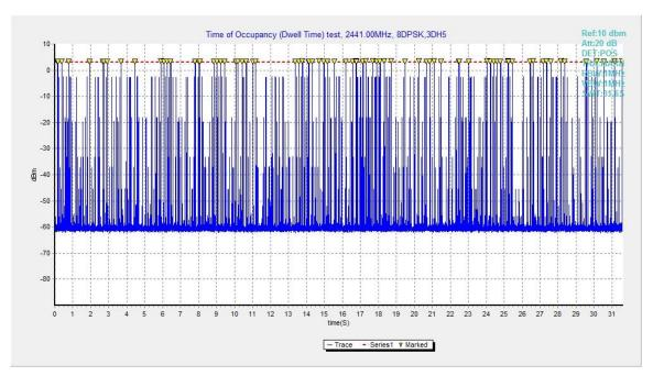
Fig.81. Number of Transmissions Measurement: Channel 39, Packet 3-DH5
