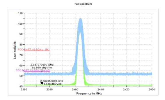
Fig.60. Radiated emission (Power):  $\pi/4$  DQPSK, low channel
