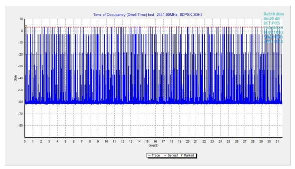
Fig.79. Number of Transmissions Measurement: Channel 39, Packet 3-DH3
