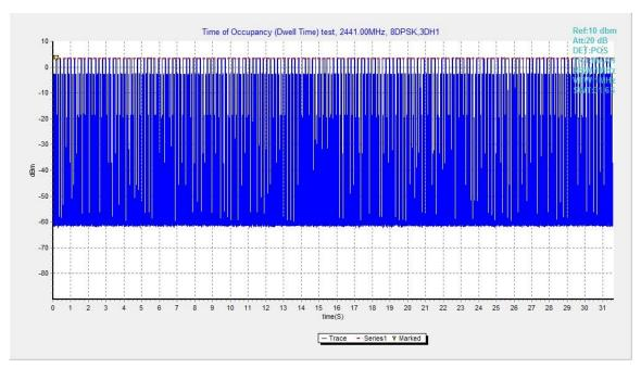
Fig.77. Number of Transmissions Measurement: Channel 39, Packet 3-DH1
