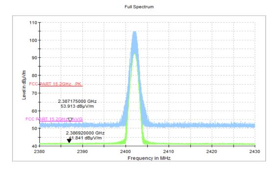
Fig.58. Radiated emission (Power): GFSK, low channel
