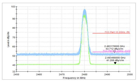
Fig.59. Radiated emission (Power) GFSK, high channel
