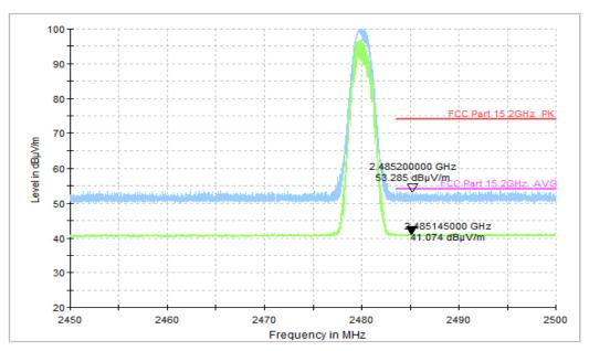
Fig.63. Radiated emission (Power): 8DPSK, high channel
