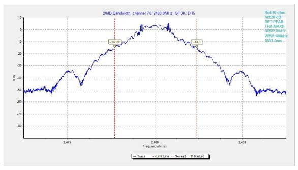
Fig.84. 20dB Bandwidth: GFSK, Channel 78
