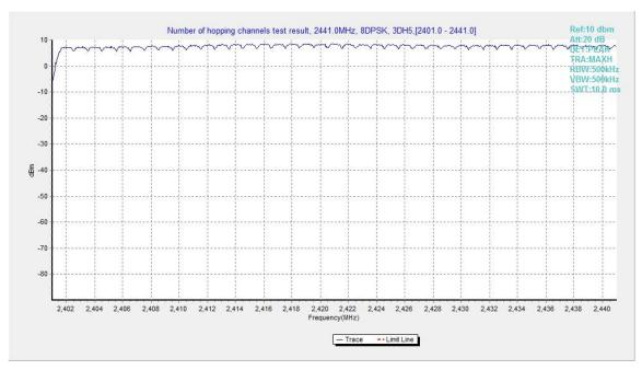
Fig.98. Number of hopping frequencies: 8DPSK, Channel 0 - 39
