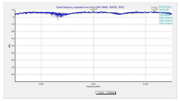
Fig.93. Carrier frequency separation measurement: 8DPSK, Channel 39
