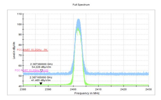
Fig.62. Radiated emission (Power): 8DPSK, low channel
