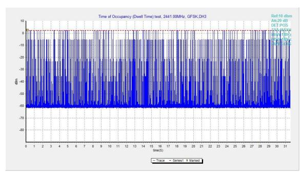
Fig.67. Number of Transmissions Measurement: Channel 39, Packet DH3
