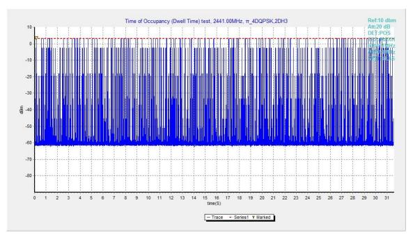
Fig.73. Number of Transmissions Measurement: Channel 39, Packet 2-DH3
