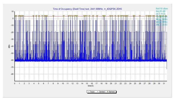
Fig.75. Number of Transmissions Measurement: Channel 39, Packet 2-DH5
