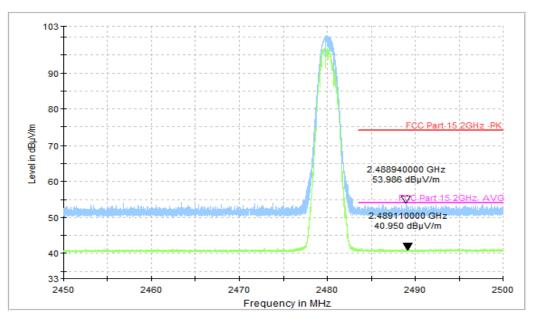
Fig.61. Radiated emission (Power):  $\pi/4$  DQPSK, high channel
