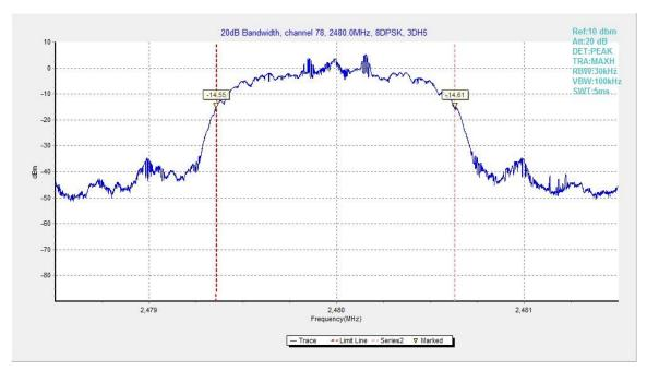
Fig.90. 20dB Bandwidth: 8DPSK, Channel 78
