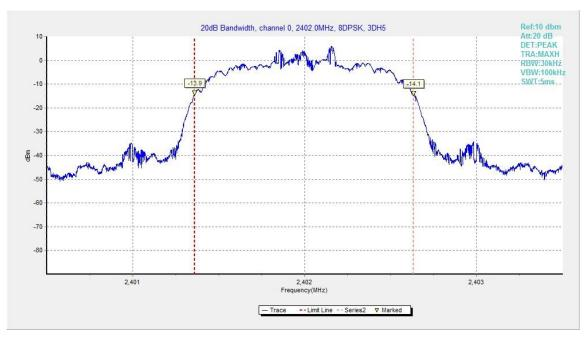
Fig.88. 20dB Bandwidth: 8DPSK, Channel 0
