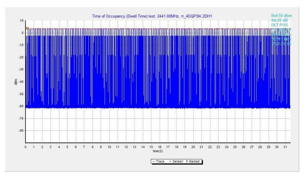
Fig.71. Number of Transmissions Measurement: Channel 39, Packet 2-DH1
