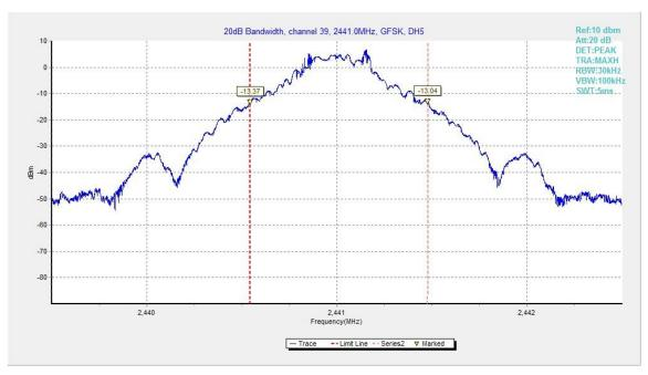
Fig.83. 20dB Bandwidth: GFSK, Channel 39
