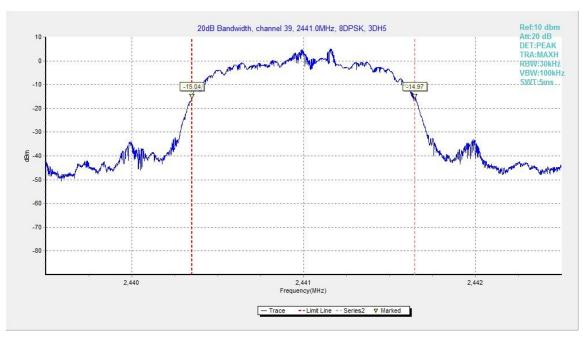
Fig.89. 20dB Bandwidth: 8DPSK, Channel 39
