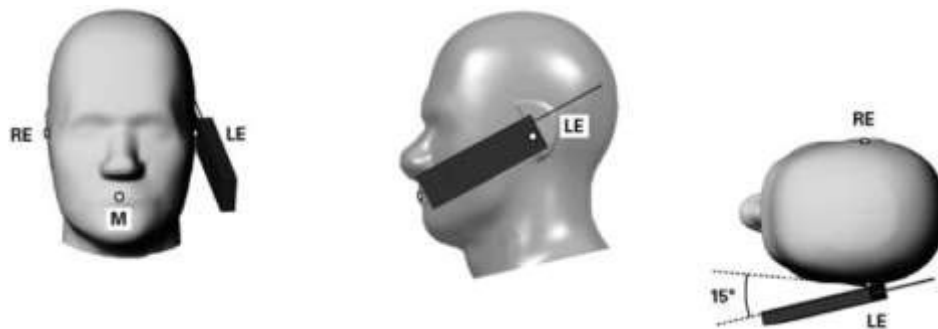
Figure 6.5. Tilt 15^\circ position of the wireless device
