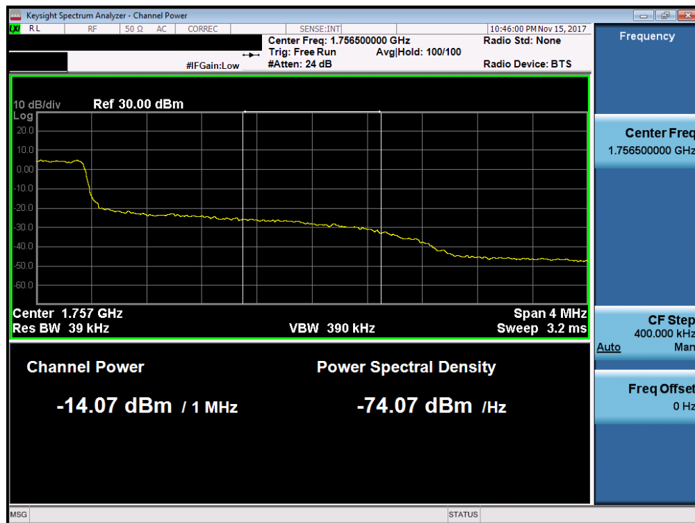
Plot 7-100. Upper Extended Band Edge Plot (Band 4 - 3.0MHz QPSK - Full RB Configuration)
