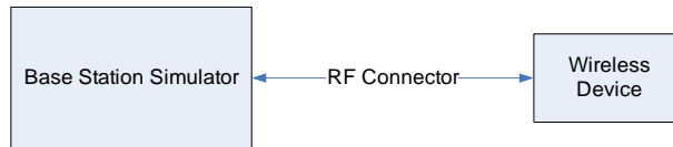
Figure 9-2 Power Measurement Setup
