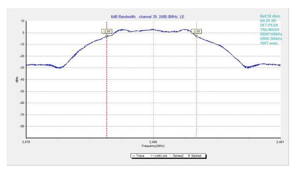
Fig.22. 6dB Bandwidth: GFSK, 2480 MHz
