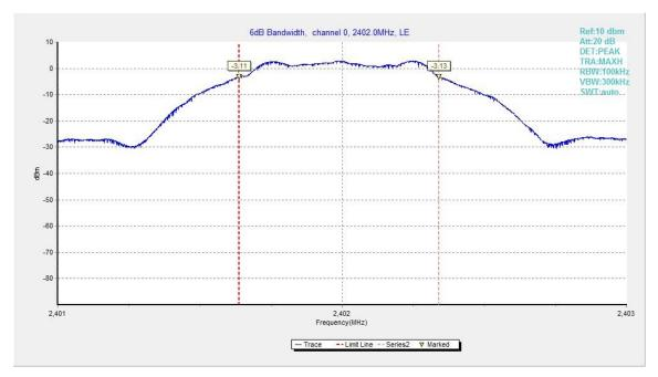
Fig.20. 6dB Bandwidth: GFSK, 2402 MHz
