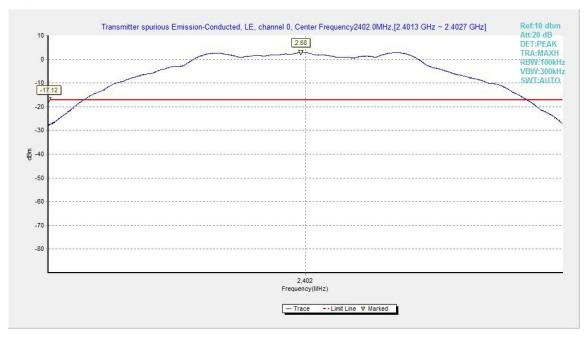
Fig.3. Transmitter Spurious Emission - Conducted: GFSK,2402MHz
