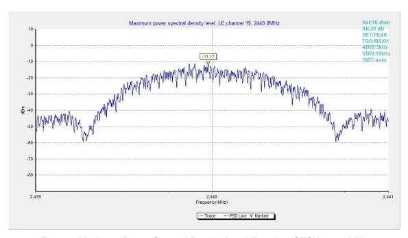
Fig.24. Maximum Power Spectral Density Level Function: GFSK, 2440 MHz
