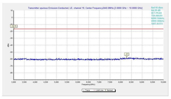
Fig.11. Transmitter Spurious Emission - Conducted: GFSK, 2440 MHz, 3GHz - 10GHz
