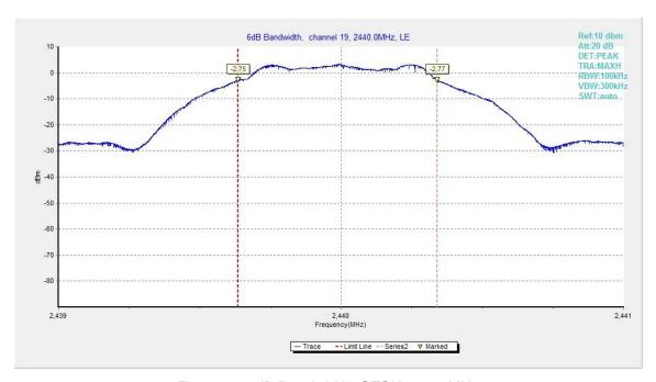
Fig.21. 6dB Bandwidth: GFSK, 2440 MHz
