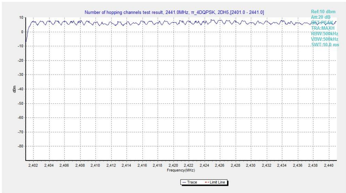
Fig.96. Number of hopping frequencies: \pi/4 DQPSK, Channel 0 - 39
