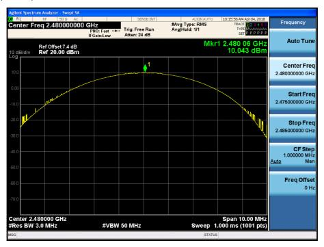
Test Plots (8DPSK) Peak Power (CH.0)
