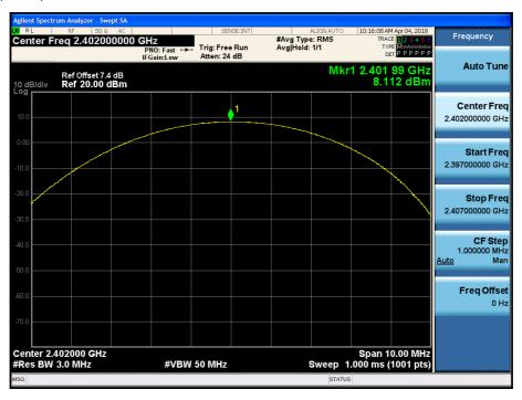
Test Plots (π/4DQPSK) Peak Power (CH.39)
