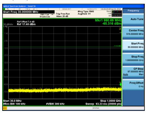
Test Plots (GFSK)- 1 GHz – 3 GHz Spurious Emission (CH.39)
