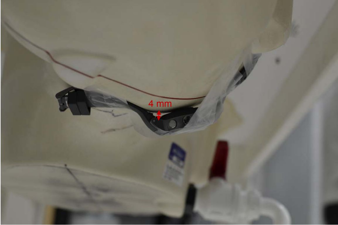
SAR Test Setup Photo 3 – Back side at 0.0 cm for Antenna 3, with gap at hinge
