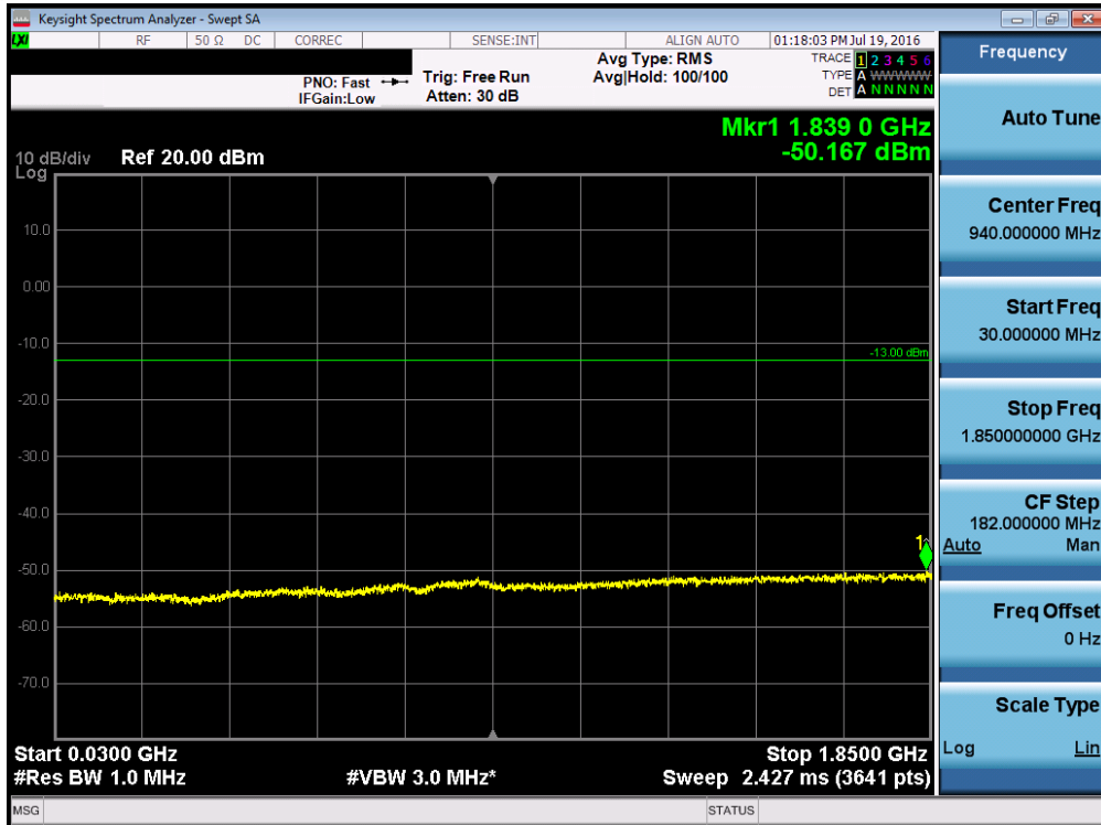
Plot 7-61. Conducted Spurious Plot (Band 2 – 10.0MHz QPSK – RB Size 1, RB Offset 0 – Mid Channel)
