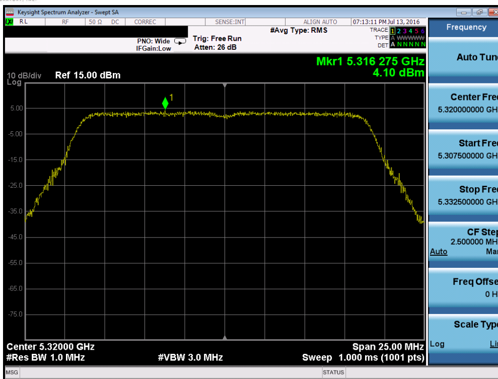
Plot 7-91. Power Spectral Density Plot (20MHz BW 802.11n (UNII Band 2A) – Ch. 64)
