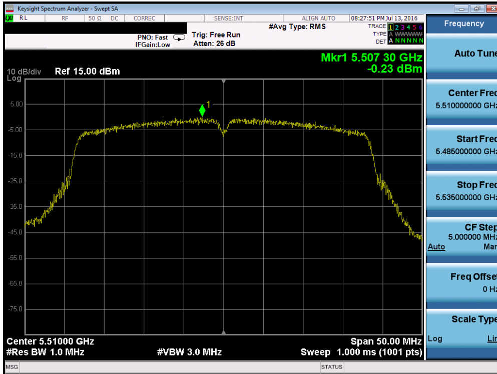
Plot 7-139. Power Spectral Density Plot (40MHz BW 802.11n (UNII Band 2C) – Ch. 102)
