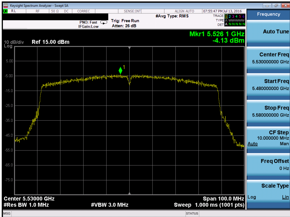
Plot 7-104. Power Spectral Density Plot (80MHz BW 802.11ac (UNII Band 2C) – Ch. 106)
