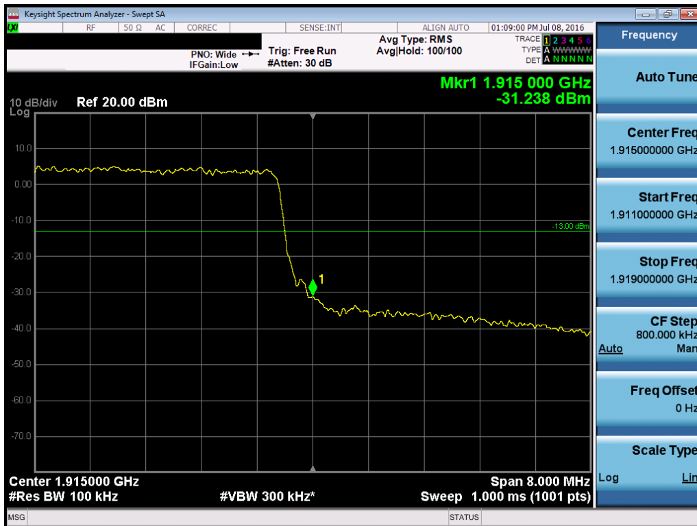
Plot 7-158. Upper Band Edge Plot (Band 2/25 – 10.0MHz QPSK – RB Size 50)
