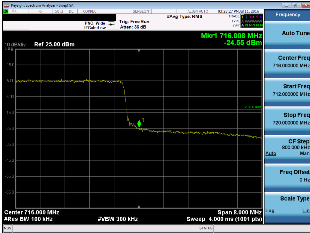
Plot 7-99. Upper Band Edge Plot (Band 12/17 – 10.0MHz QPSK – RB Size 50)
