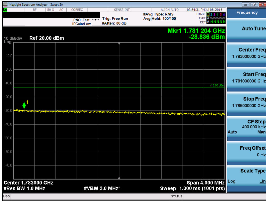
Plot 7-143. Upper Extended Band Edge Plot (Band 66 – 20.0MHz QPSK – RB Size 100)
