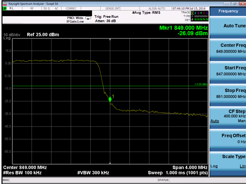
Plot 7-113. Upper Band Edge Plot (Band 5 – 5.0MHz QPSK – RB Size 25)
