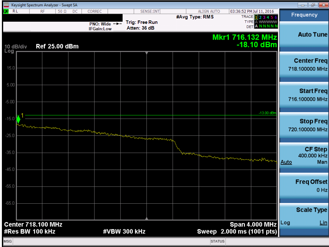
Plot 7-95. Upper Extended Band Edge Plot (Band 12 – 3.0MHz QPSK – RB Size 15)
