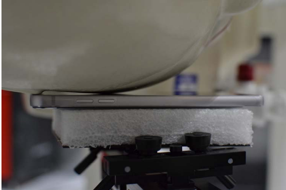
SAR Test Setup Photo 1: Right Cheek
