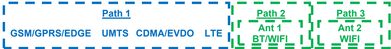
Figure 1-1 Simultaneous Transmission Paths
