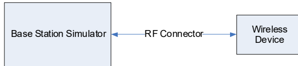
Figure 9-3 Power Measurement Setup
