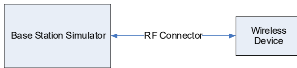
Figure 9-4 Power Measurement Setup
