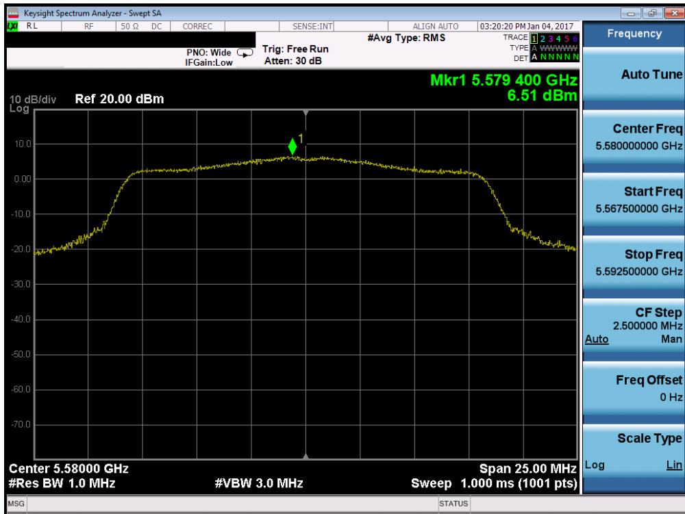
Plot 7-134. Power Spectral Density Plot (802.11a (UNII Band 2C) – Ch. 116)
