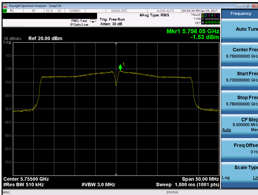
Plot 7-150. Power Spectral Density Plot (40MHz BW 802.11n (UNII Band 3) – Ch. 151)
