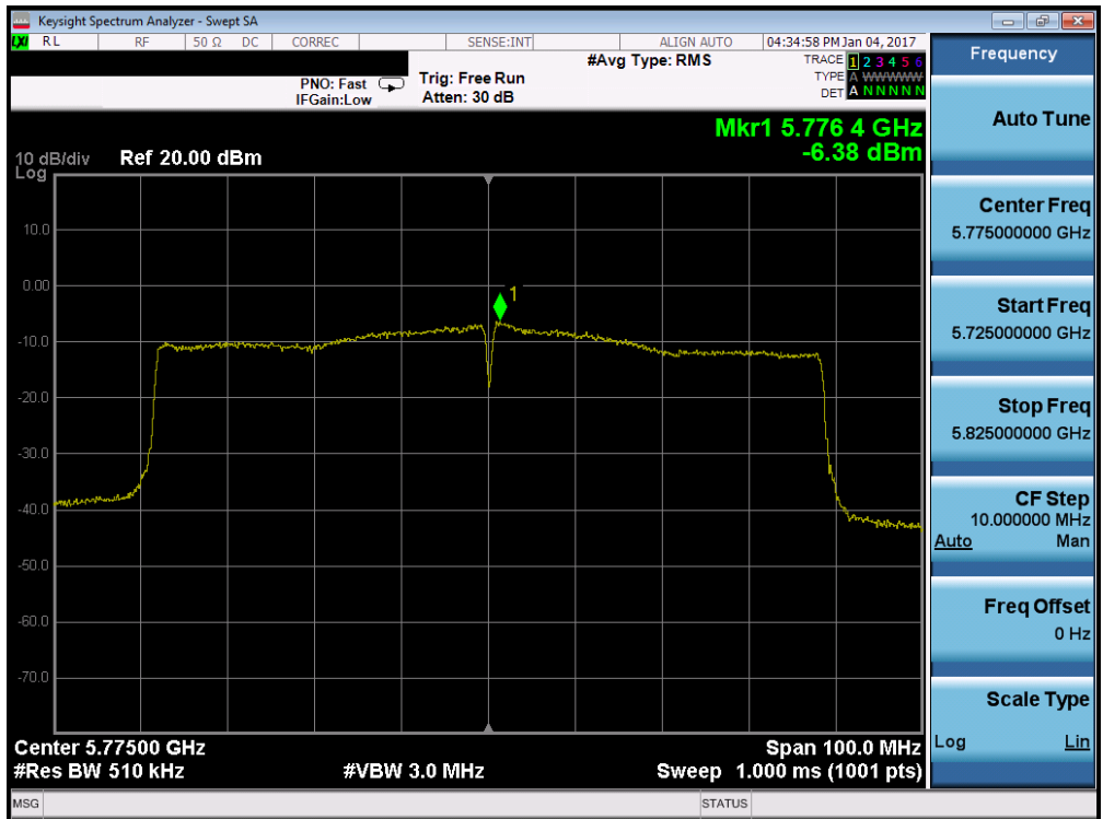
Plot 7-152. Power Spectral Density Plot (80MHz BW 802.11ac (UNII Band 3) – Ch. 155)
