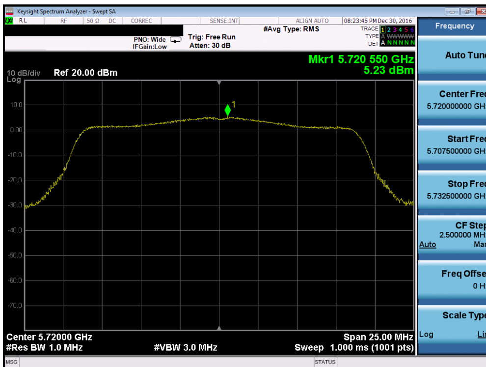
Plot 7-100. Power Spectral Density Plot (20MHz BW 802.11n (UNII Band 2C) – Ch. 144)
