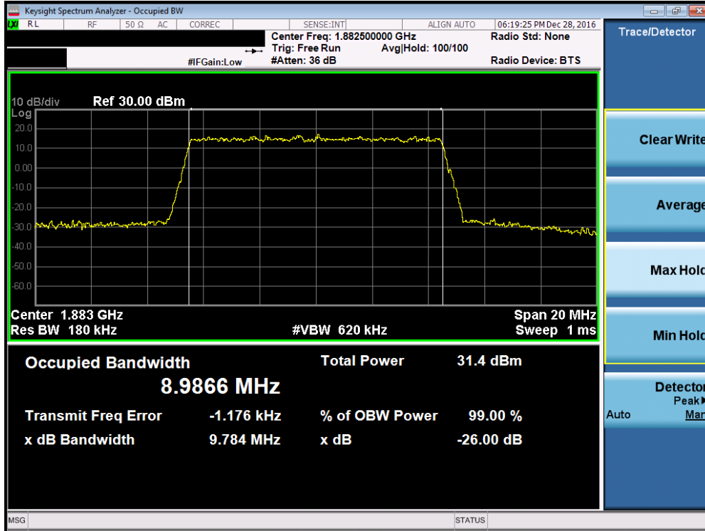
Plot 7-59. Occupied Bandwidth Plot (Band 2/25 – 10.0MHz 16-QAM – RB Size 50)
