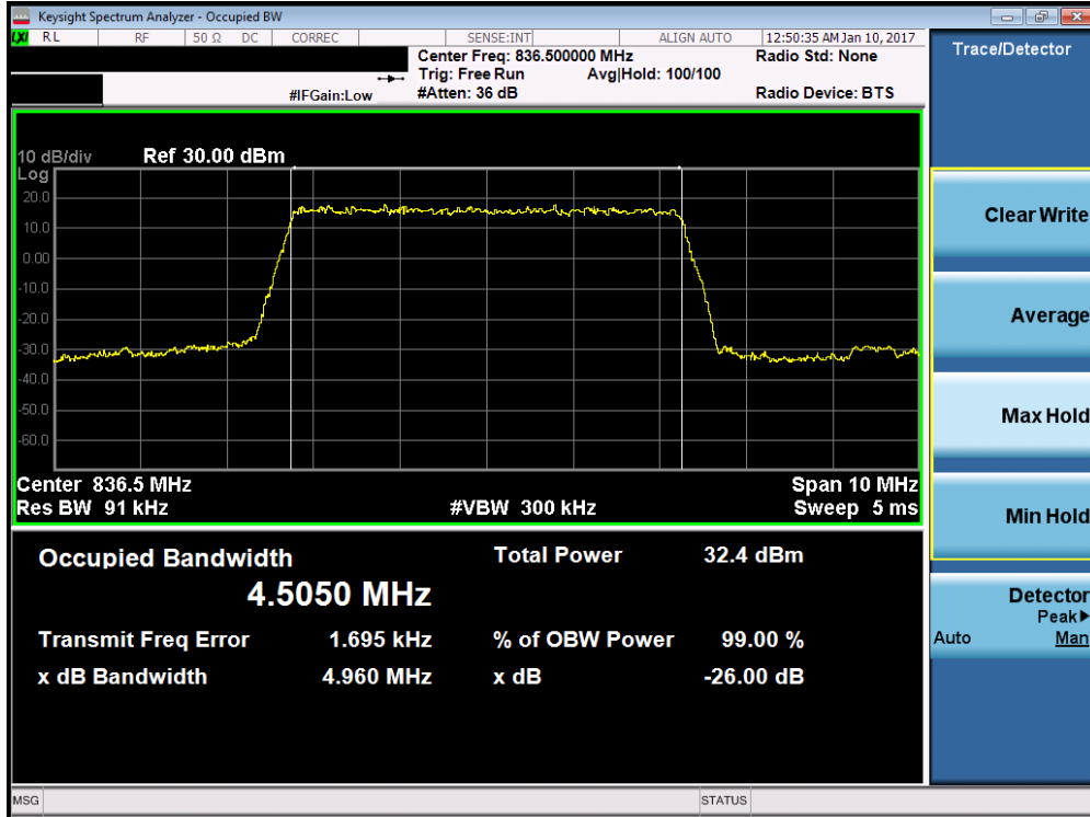
Plot 7-25. Occupied Bandwidth Plot (Band 5 – 5.0MHz QPSK – RB Size 25)
