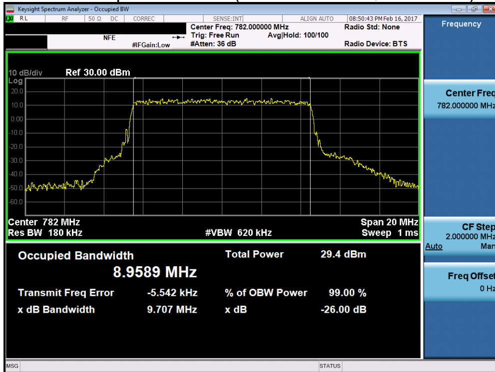
Plot 7-18. Occupied Bandwidth Plot (Band 13 – 10.0MHz 64-QAM – RB Size 50)
