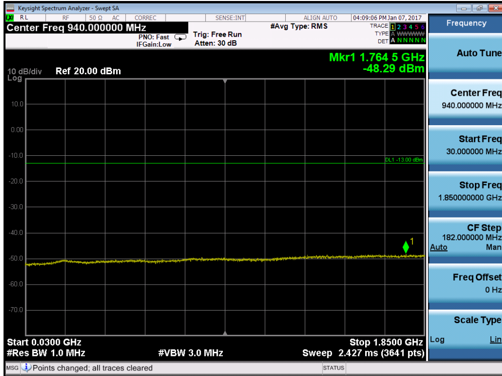
Plot 7-70. Conducted Spurious Plot (PCS WCDMA Mode – Ch. 9538)
