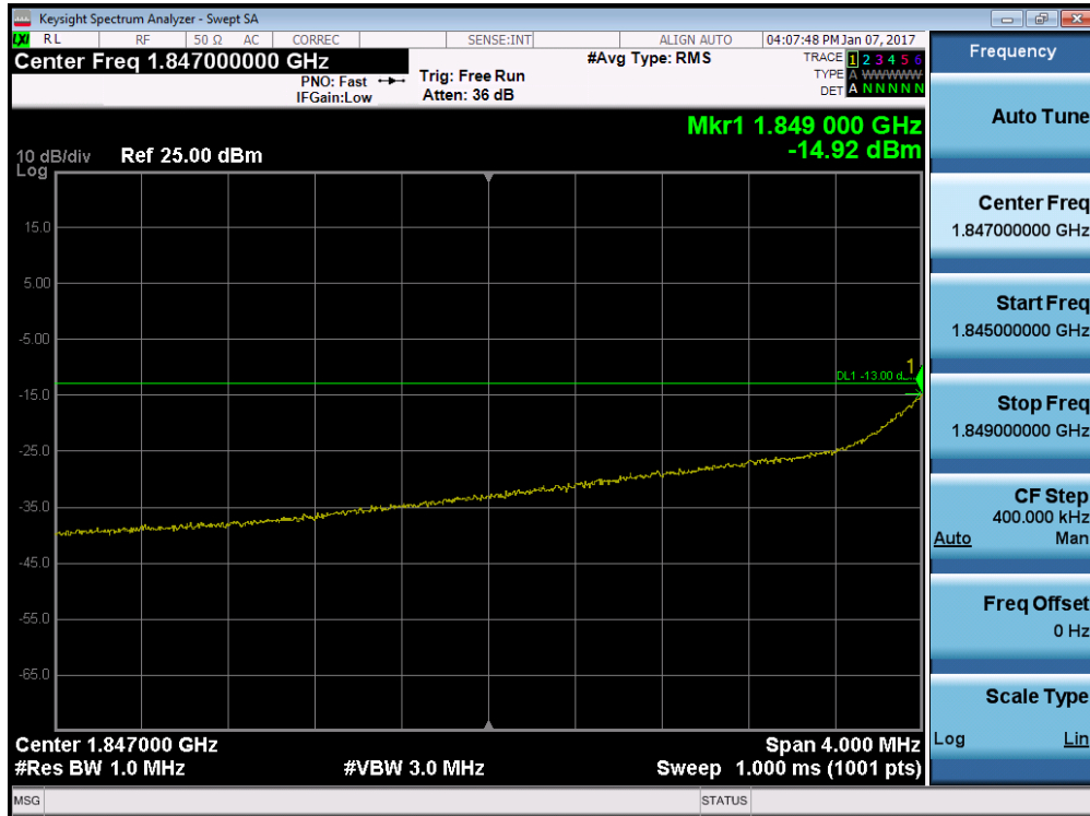
Plot 7-94. 4MHz Span Plot (PCS WCDMA Mode – Ch. 9262)
