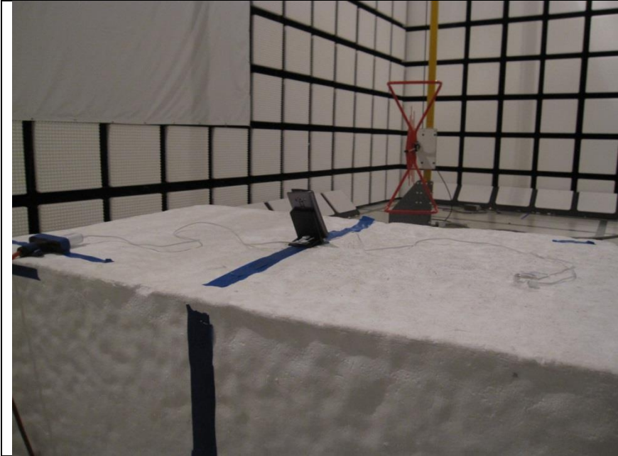
RADIATED BACK PHOTO W/ SMARTCOVER + DOCK (BELOW 1 GHz)
