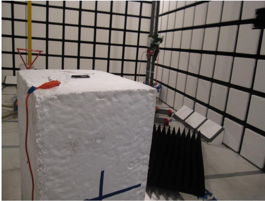
RADIATED BACK PHOTO (ABOVE 1 GHz)
