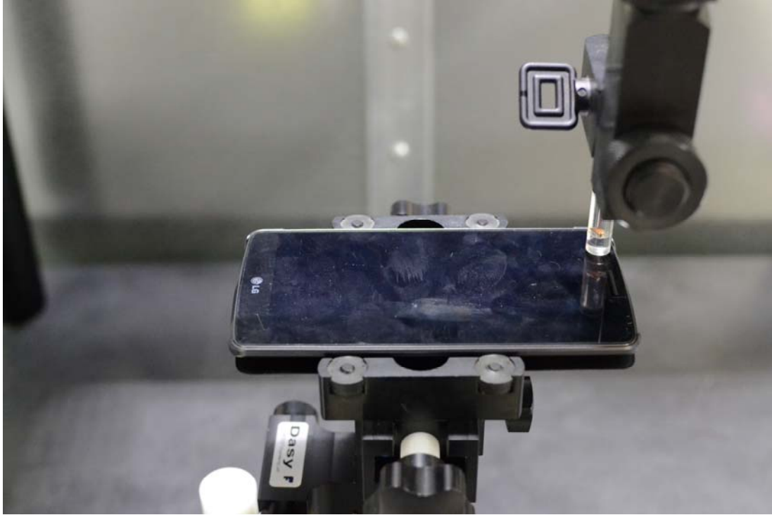
Figure 13-3 Test Setup for Wireless Device (Wireless Charging Cover – Open)
