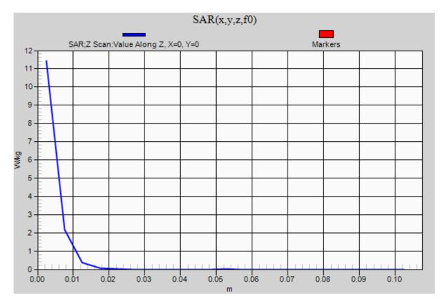
Frequency: 836.6 MHz; Duty Cycle: 1:8; Room Ambient Temperature: 24.0°C; Liquid Temperature: 23.0°C Medium parameters used (interpolated): f = 836.6 MHz;  $\sigma = 0.91$  S/m;  $\epsilon_r = 40.661$ ;  $\rho = 1000$  kg/m<sup>3</sup> DASY5 Configuration:
