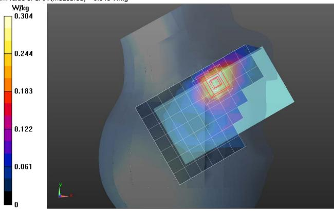
Frequency: 1908.75 MHz; Duty Cycle: 1:1; Room Ambient Temperature: 24.0°C; Liquid Temperature: 23.0°C Medium parameters used (interpolated): f = 1908.75 MHz;  $\sigma = 1.583$  S/m;  $\epsilon_r = 52.722$ ;  $\rho = 1000$  kg/m<sup>3</sup> DASY5 Configuration:
