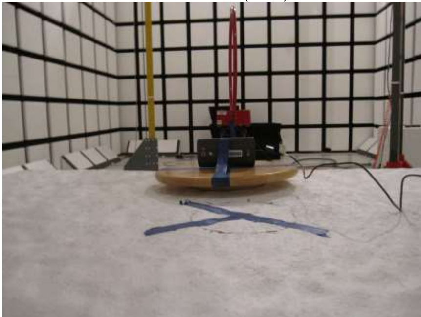
RADIATED EMISSIONS BELOW 30MHz (BACK)
