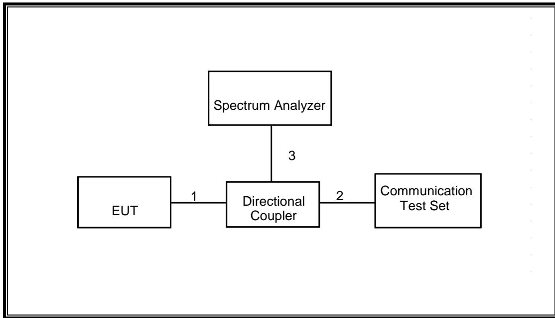
**SETUP DIAGRAM FOR RF RADIATED TESTS**
