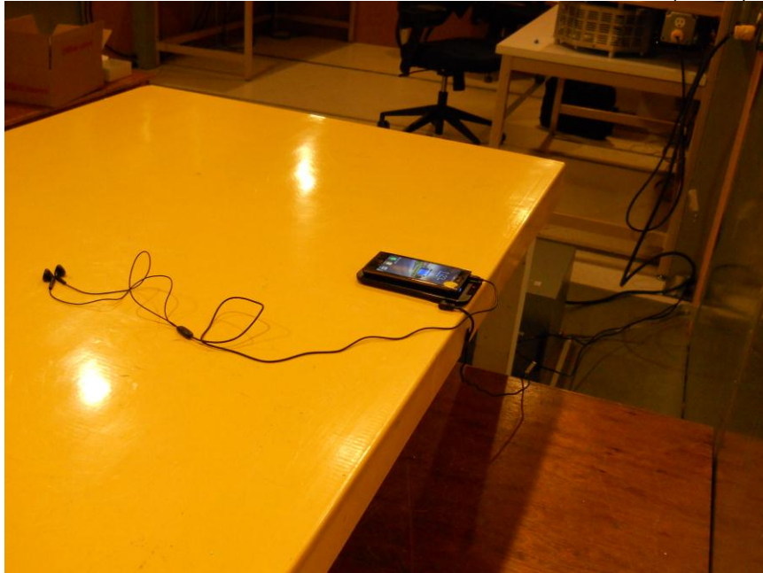
LINE CONDUCTED EMISSION WITH INDUCTIVE CHARGER (BACK)
