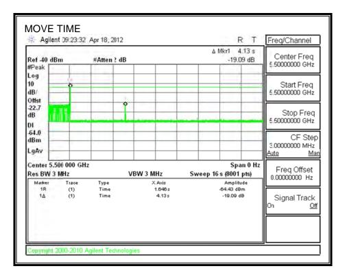
Note: The manufacturer has attested that spike after radar is a control signal and not normal traffic. Additional close-up observations show that the observed signal has a different pattern than the normal traffic.
