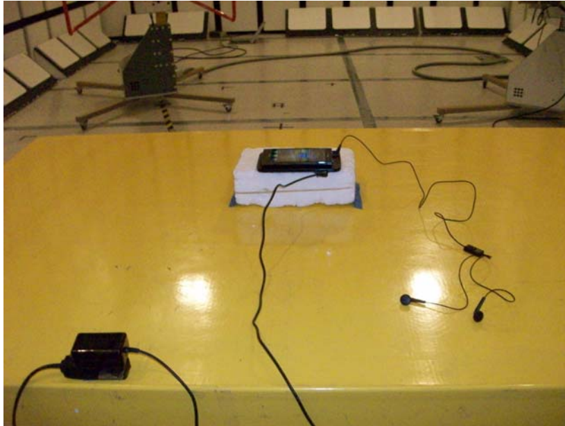
EUT ON INDUCTIVE CHARGER PAD PHOTO
