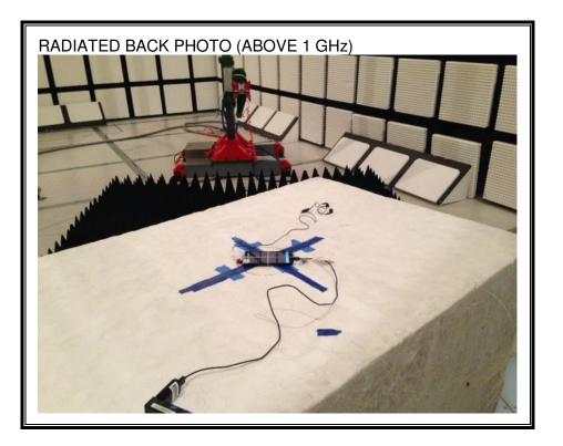
RADIATED RF MEASUREMENT SETUP FOR PORTABLE CONFIGURATION
