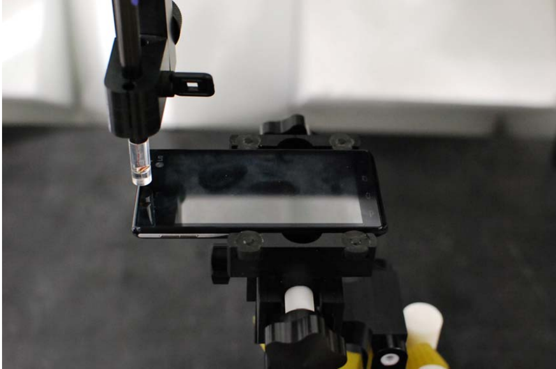
Figure 13-1 Test Setup for Wireless Device
