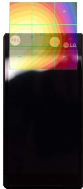
Figure 17-5 H-Field WD Scan overlay
