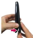
2. Remove the battery from the battery compartment by lifting the bottom of the battery using the fingertip cutout.
