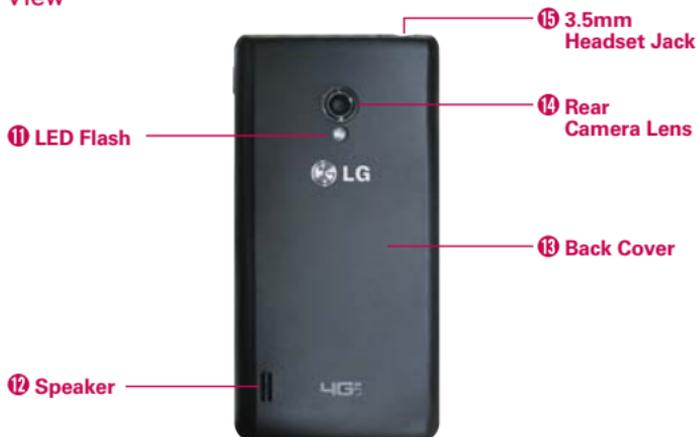
11. **LED Flash** Brightens up the captured image or recorded video when you turn on the flash.
