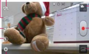
**Mode Switch** – Touch this icon to switch between Camera mode and Video mode.
