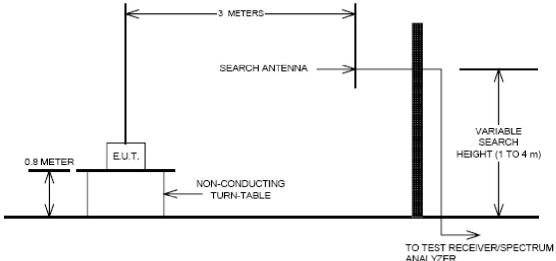
The measurement facilities used for this test have been documented in previous filings with the commission pursuant to section § 2.948. The SAC(Semi-Anechoic Chamber) meets requirements in ANSI C63.4 –2003. A mast capable of lifting the receiving antenna from a height of one to four meters is used together with a rotatable styrofoam platform mounted at three from the antenna mast.
