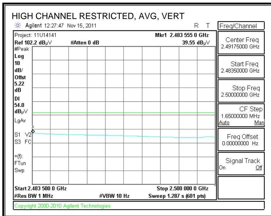
**HARMONICS AND SPURIOUS EMISSIONS****High Frequency Measurement**
