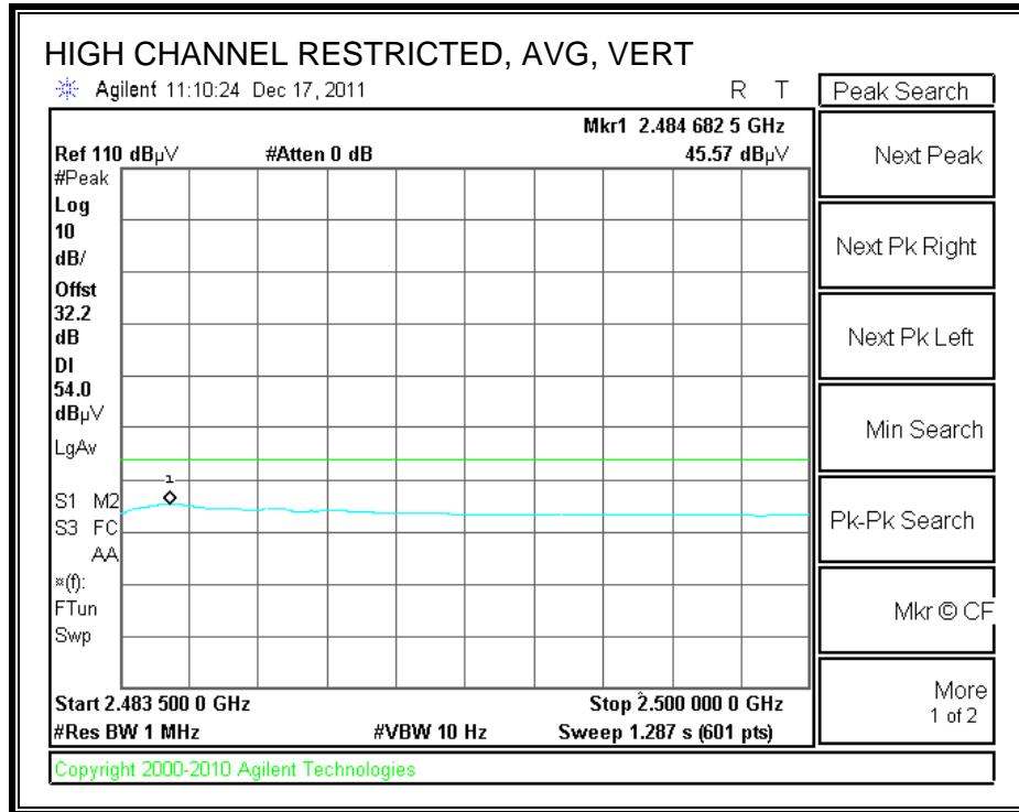
**HARMONICS AND SPURIOUS EMISSIONS****High Frequency Measurement**
