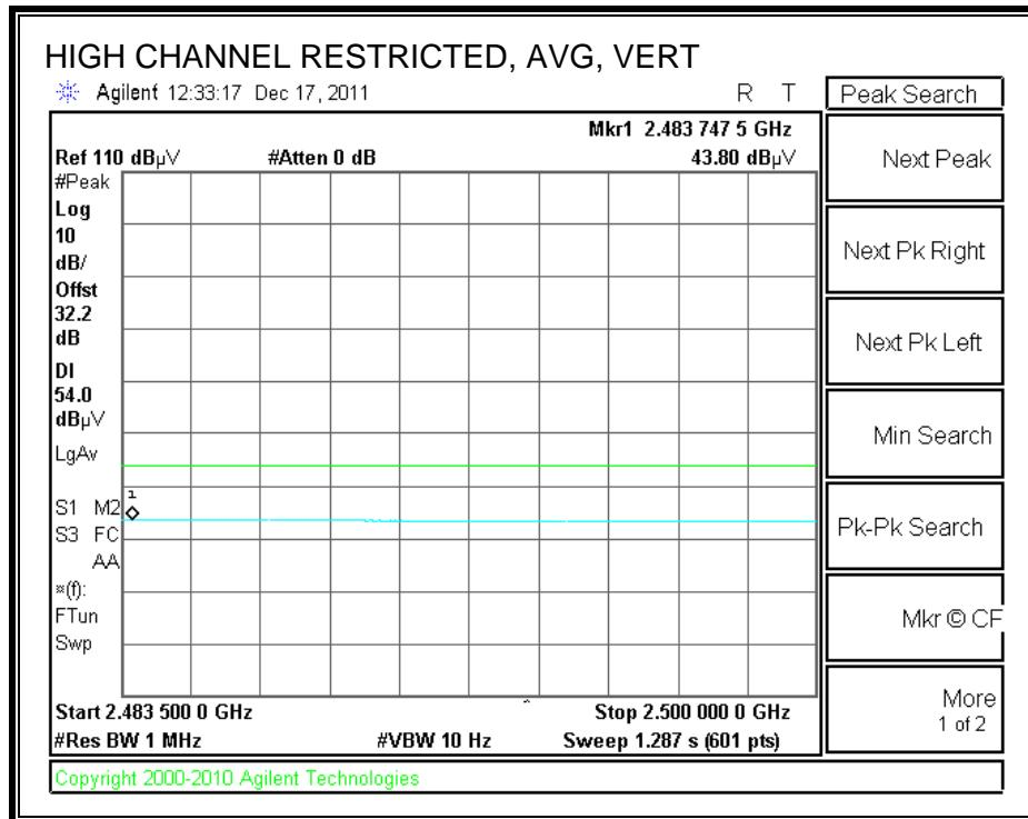
**HARMONICS AND SPURIOUS EMISSIONS****High Frequency Measurement
