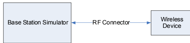
Figure 9-3 Power Measurement Setup
