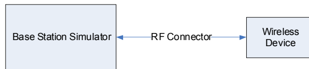
Figure 9-1 Power Measurement Setup
