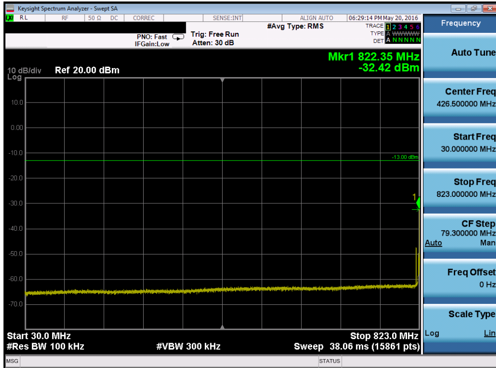
Plot 7-46. Conducted Spurious Plot (Band 5 – 5.0MHz QPSK – RB Size 1, RB Offset 0 – Low Channel)
