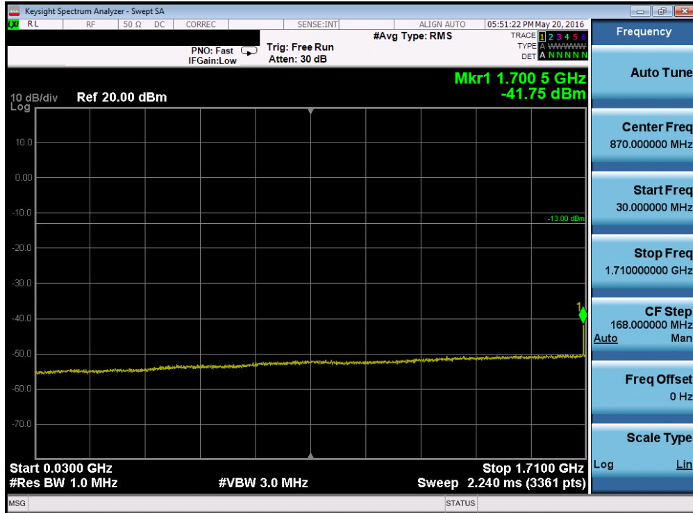
Plot 7-61. Conducted Spurious Plot (Band 4 – 20.0MHz QPSK – RB Size 1, RB Offset 0 – High Channel)
