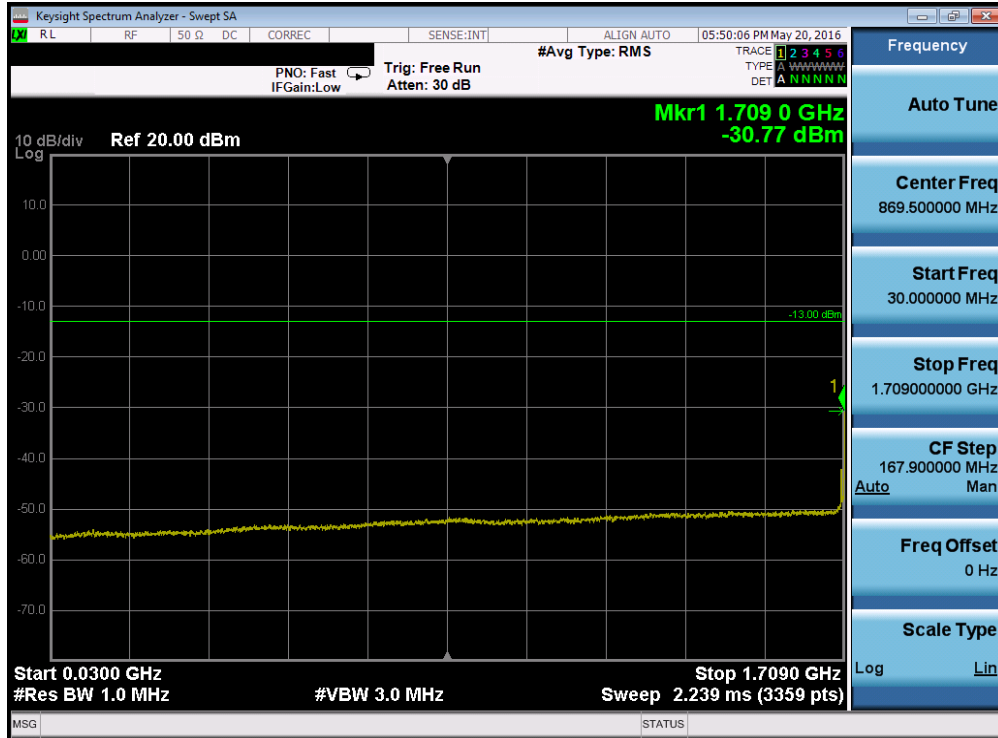
Plot 7-55. Conducted Spurious Plot (Band 4 – 20.0MHz QPSK – RB Size 1, RB Offset 0– Low Channel)
