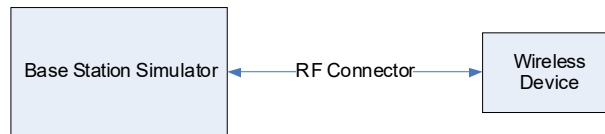
Figure 9-1 Power Measurement Setup
