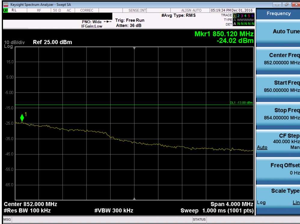
Plot 7-82. Upper Extended Band Edge Plot (Band 5 – Band 5 – 3.0MHz QPSK – RB Size 15)
