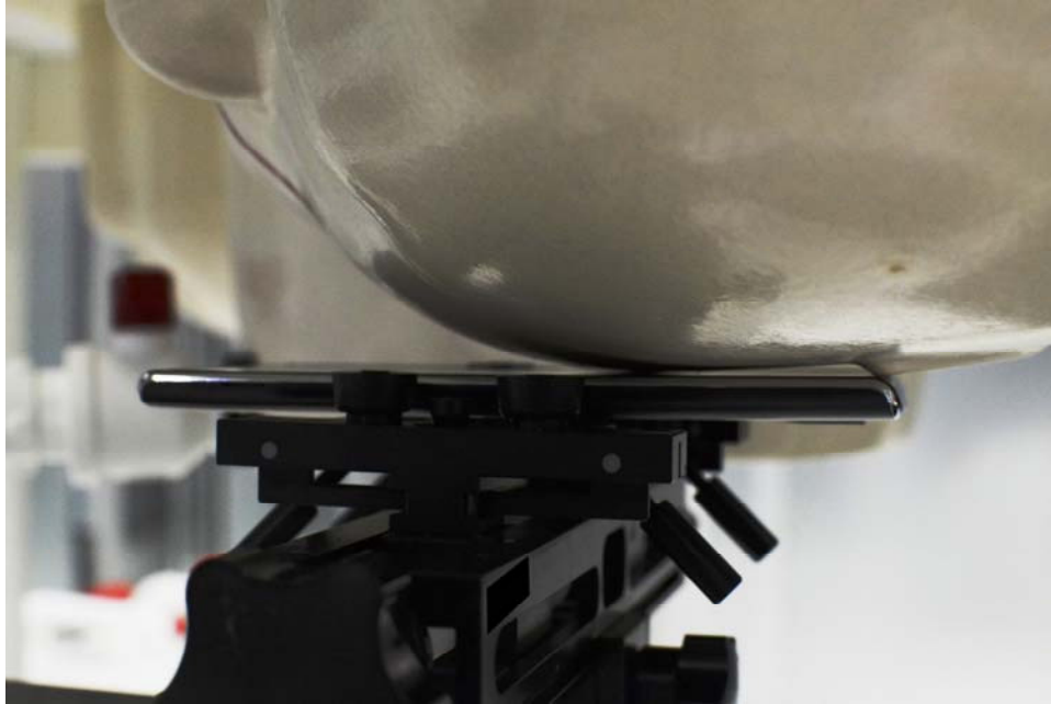
SAR Test Setup Photo 3 – Left Cheek
