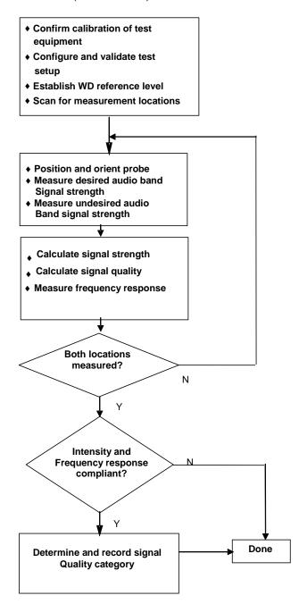
Figure 5-16 C63.19 T-Coil Signal Test Process
