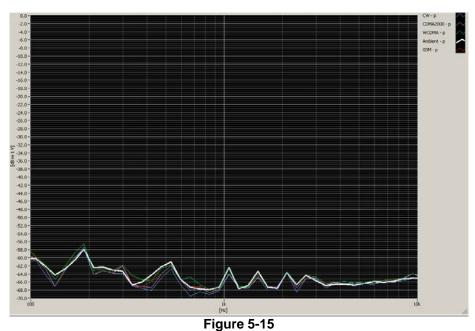
High power RF Emissions Effect with HAC Dipole on the T-coil Probe System 10mm between dipole maximum and magnetic probe
