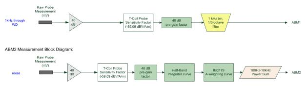
Figure 5-6 Magnetic Measurement Processing Steps
