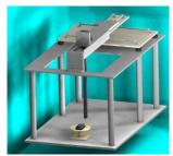
**Figure 5-3** RF Near-Field Scanner
