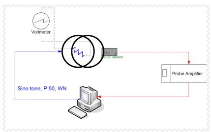
Figure 5-1 Validation Setup with Helmholtz Coil
