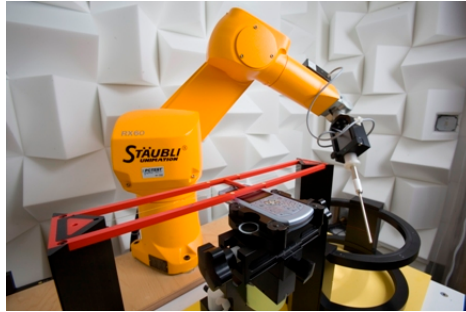
Figure 5-3 SPEAG Robotic System
