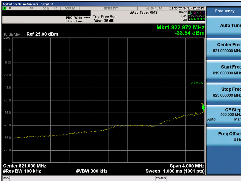
Plot 7-85. Lower Extended Band Edge Plot (Band 5 – 1.4MHz QPSK – RB Size 6)
