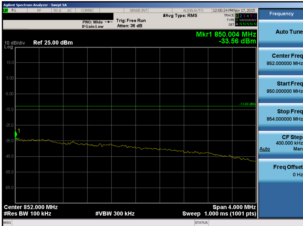
Plot 7-91. Upper Extended Band Edge Plot (Band 5 – Band 5 – 3.0MHz QPSK – RB Size 15)
