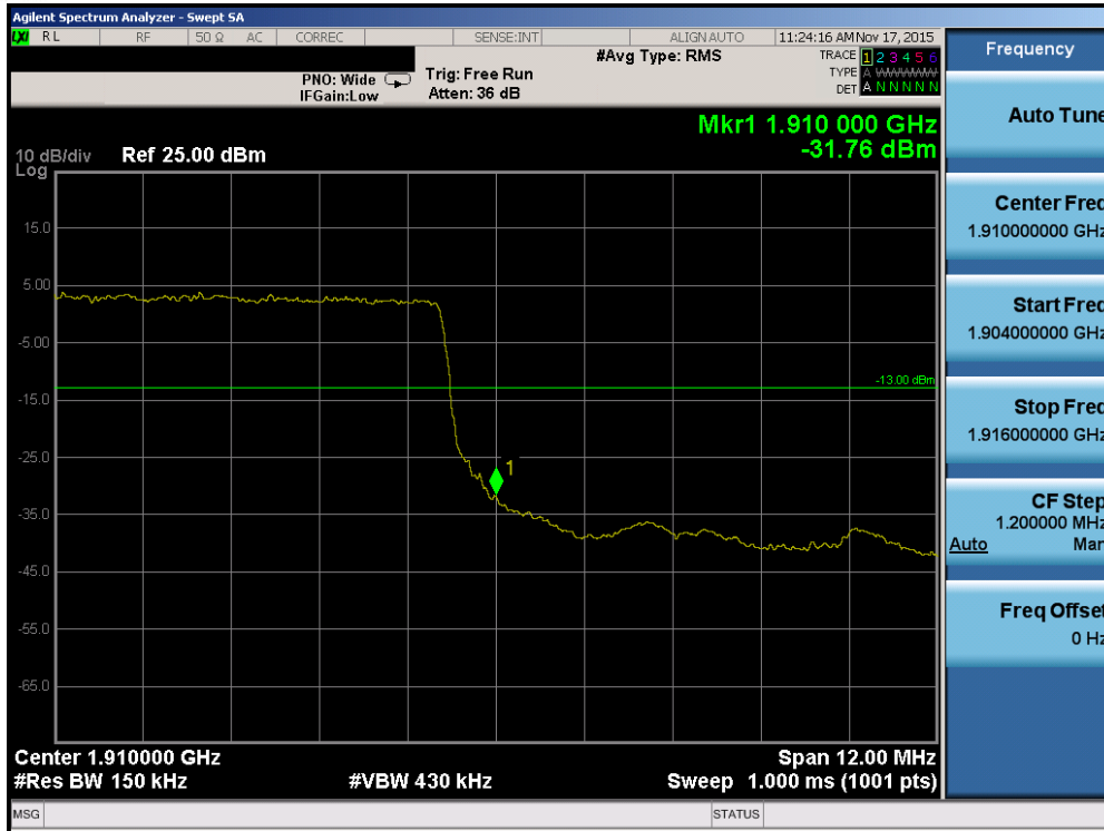
Plot 7-140. Upper Band Edge Plot (Band 2 – 15.0MHz QPSK – RB Size 75)
