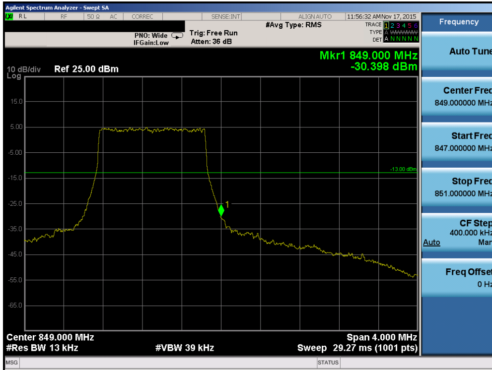
Plot 7-86. Upper Band Edge Plot (Band 5 – 1.4MHz QPSK – RB Size 6)
