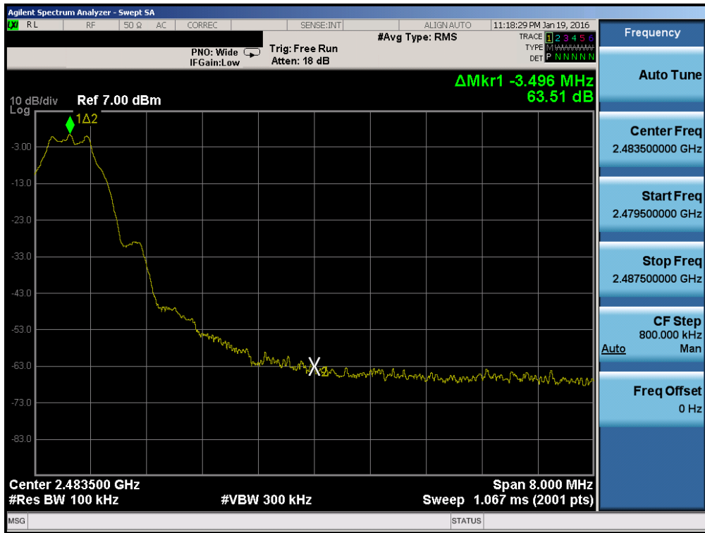
Plot 7-11. Band Edge Plot (Bluetooth (LE) – Ch. 39)
