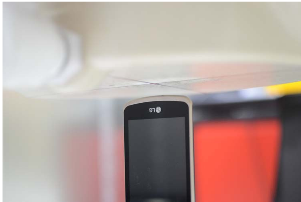
SAR Test Setup Photo 8: Bottom Edge 1.0 cm
