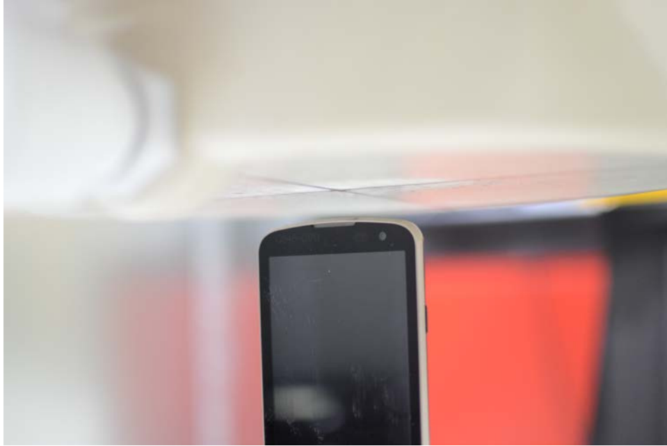
SAR Test Setup Photo 7: Top Edge 1.0 cm
