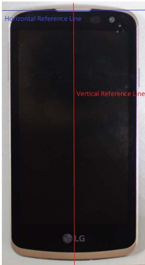
SAR Test Setup Photo 11: Vertical and Horizontal Reference Lines
