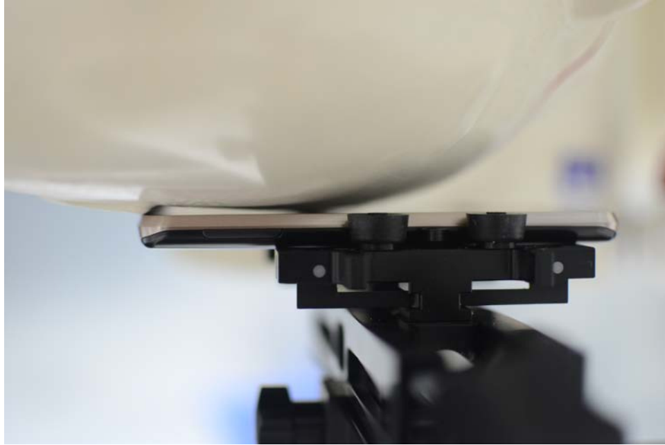
SAR Test Setup Photo 1: Right Cheek
