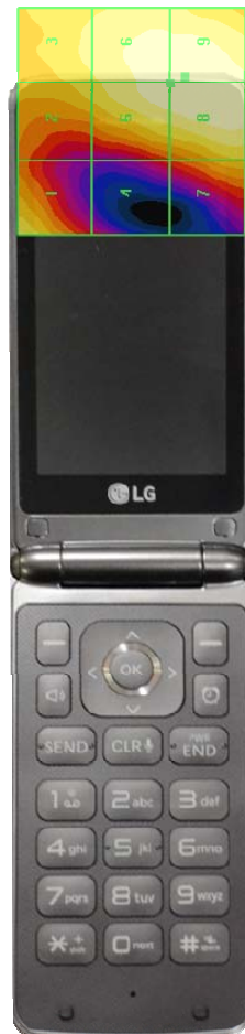
Figure 18-4 E-Field WD Scan overlay
