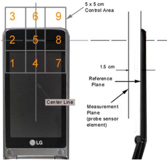
Figure 18-3 5x5 Scan grid above WD
