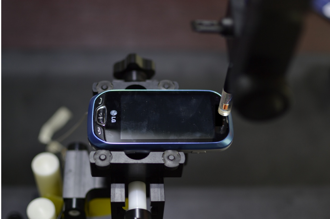
Figure 13-1 Test Setup for Wireless Device
