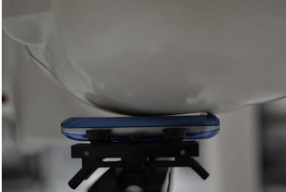
SAR Test Setup Photo 3: Left Cheek
