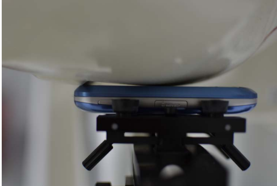
SAR Test Setup Photo 1: Right Cheek
