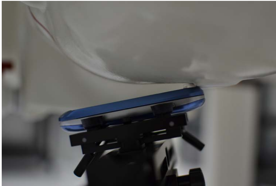
SAR Test Setup Photo 4: Left Tilt
