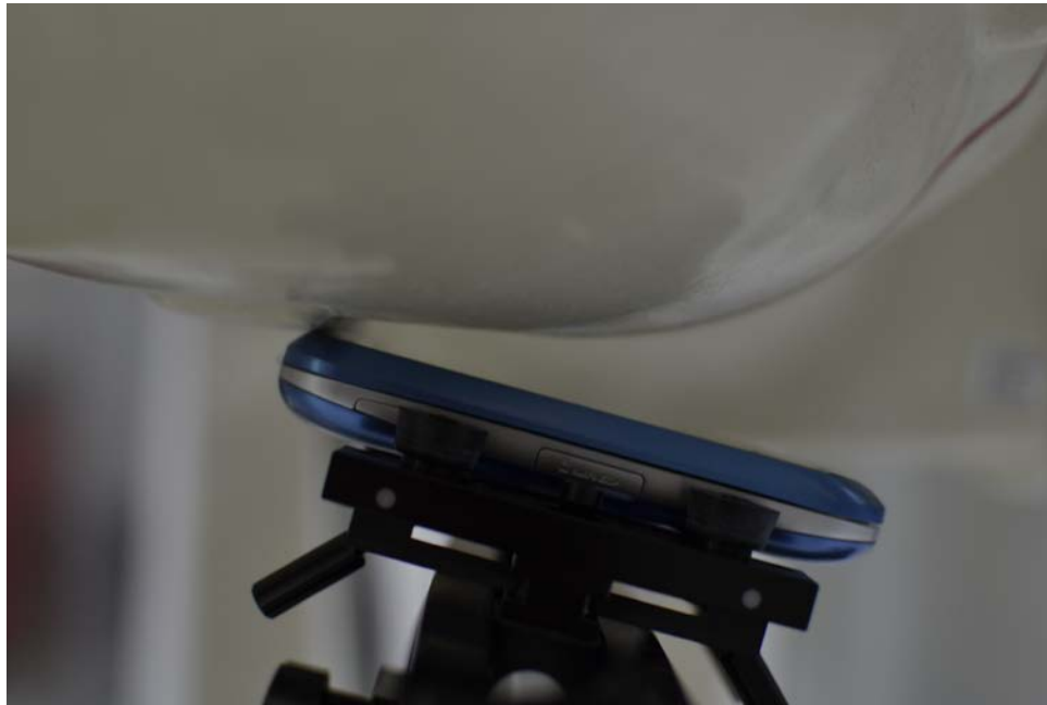
SAR Test Setup Photo 2: Right Tilt
