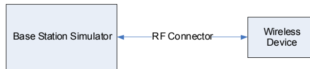
Figure 8-1 Power Measurement Setup
