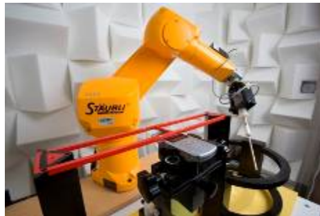
Figure 5-5 SPEAG Robotic System
