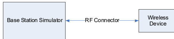
Figure 9-2 Power Measurement Setup
